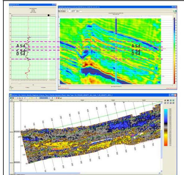
Figure 6: Upper: Pseudo density from multiattribute inversion at a calibration well. Lower: Map of sand distribution for a particular sand body.
