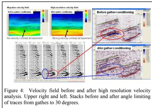
Figure 4: Velocity field before and after high resolution velocity analysis. Upper right and left. Stacks before and after angle limiting of traces from gathers to 30 degrees.
