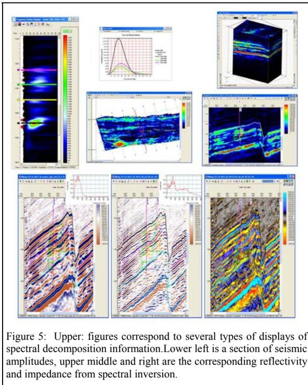
Figure 5: Upper: figures correspond to several types of displays of spectral decomposition information. Lower left is a section of seismic amplitudes, upper middle and right are the corresponding reflectivity and impedance from spectral inversion.
