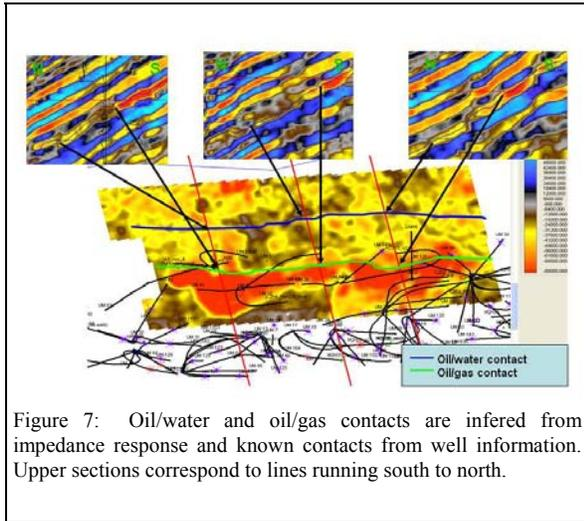
Figure 7: Oil/water and oil/gas contacts are inferred from impedance response and known contacts from well information. Upper sections correspond to lines running south to north.
