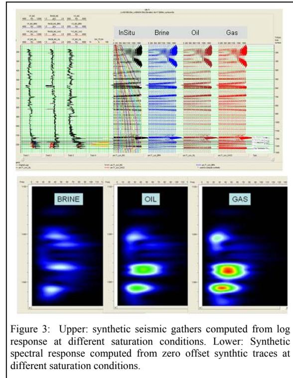
Figure 3: Upper: synthetic seismic gathers computed from log response at different saturation conditions. Lower: Synthetic spectral response computed from zero offset synthetic traces at different saturation conditions.
