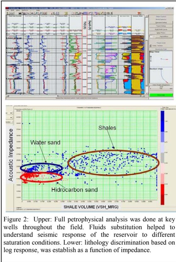
Figure 2: Upper: Full petrophysical analysis was done at key wells throughout the field. Fluids substitution helped to understand seismic response of the reservoir to different saturation conditions. Lower: lithology discrimination based on log response, was established as a function of impedance.
