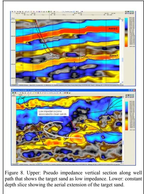
Figure 8. Upper: Pseudo impedance vertical section along well path that shows the target sand as low impedance. Lower: constant depth slice showing the aerial extension of the target sand.
