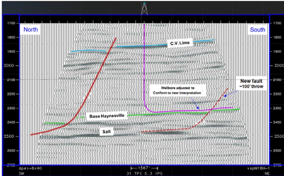
*Interpretation of the final time-domain image showing the location of the target Base Haynesville and the new fault that was interpreted to intersect the planned wellbore.*
