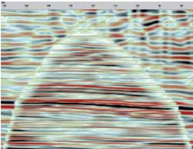
**Figure 1** This image shows 3D BSI inside 3D surface seismic. Note the significantly higher resolution of the BSI data.
