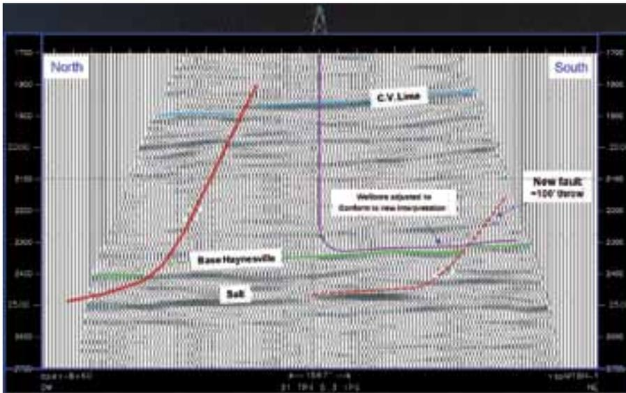
**Figure 2** Interpretation of the final time-domain image showing the location of the target Base Haynesville and the new fault that was interpreted to intersect the planned wellbore.
