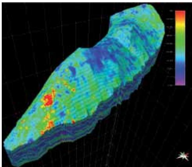
**Figure 3** 3D distribution of Brittleness in the Steele and Niobrara shale at Teapot Dome, derived from the Extended Elastic Inversion.
