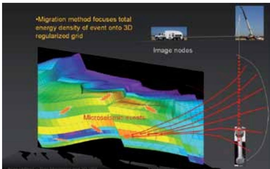
**Figure 4** In a dynamic subsurface model integrating production information, this diagram shows SIGMA<sup>3</sup> Microseismic technology using a full 3D anisotropic velocity model for microseismic processing.
